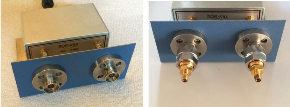
Left image: The APC-7 to 3.5mm female flange fitted to the VNWA with two SMA male-male adaptors. Right image: The VNWA ready for calibration and measurements of the male female SMA adaptors.
