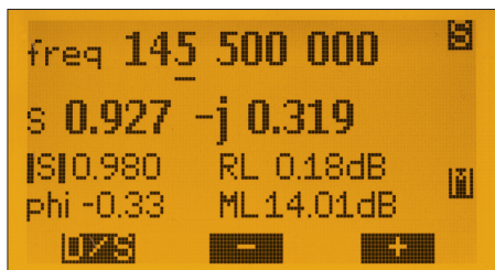
Fig. 17: Single frequency measurement of the Reflection coefficient
