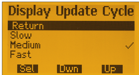
Fig. 28: The display repetition rate can be set to Slow , Medium or Fast .
