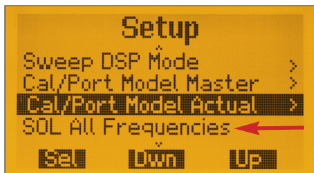
Fig. 12: Starting point of the master calibration
