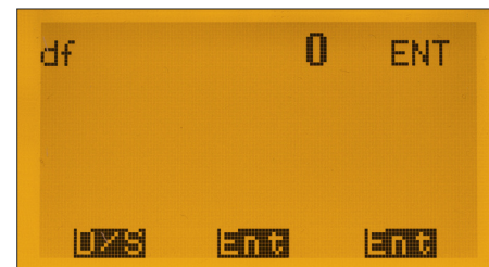
Fig. 30: Input option for the correction of the frequency offset
