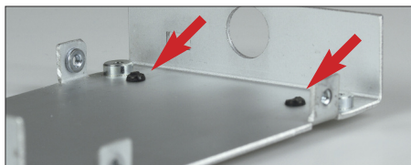
Fig. 9: Cut rubber feet after insertion into the housing
