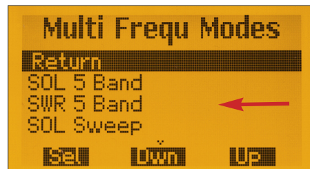
Fig. 19: Additional current calibration option for the mode SWR 5 frequencies
