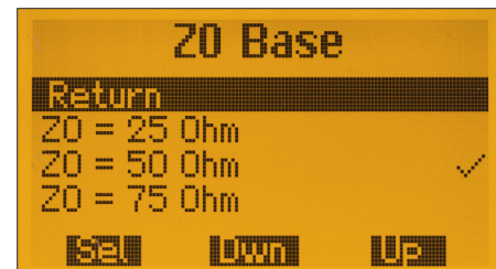
Fig 30a: Selection options for the Reference impedance basis
