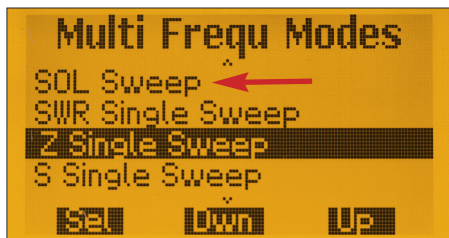
Fig. 11a: SOL compensation for the actual Frequencies for a multi-frequency measurement
