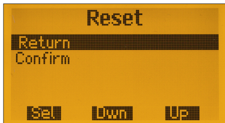
Fig. 33: This menu allows reset to the factory settings.
