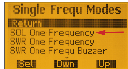
Fig. 11: Menu item for SOL compensation for the actual frequency
