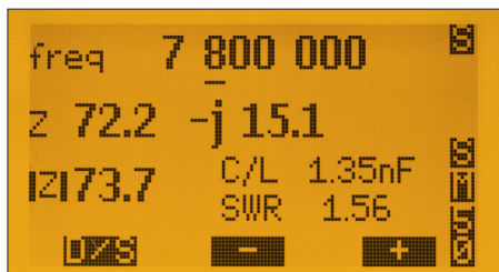
Fig. 16: Single frequency measurement of Impedance
