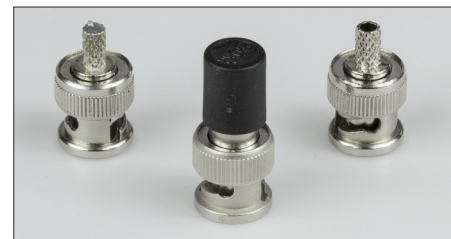
Fig. 10: The kit contains a set of calibration elements for use in the frequency range up to about 100 MHz, consisting of a 50\ \Omega Termination from Telegärtner (centre) and two BNC coaxial cable connector for making the Short and Open reference elements (see text).
