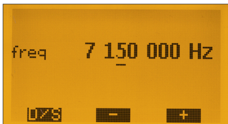
Fig. 21: Screen display when operating the FA-VA5 as an RF generator
