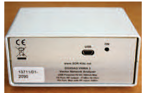
PHOTO 2: Rear panel of the VNWA3 showing the mini USB connector and the red power LED.
