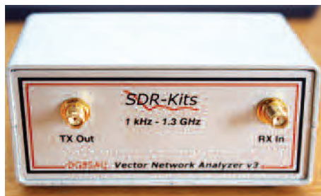
PHOTO 1: The front panel of the VNWA3 with transmit (TX) connector of the left and receive (RX) connector of the right.
