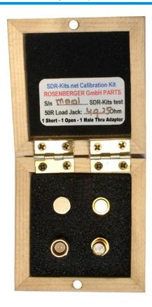
The DC Resistance value of the Load is measured by SDR-Kits by a 4 point Testbox, comparing to 0.01% 50 ohm. Enter this value in Calibration Settings
