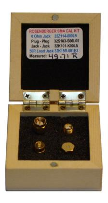
The DC Resistance value of the Load is measured by SDR-Kits by a 4 point testbox, comparing to 0.01% 50 ohm. Enter this value in Calibration Settings
