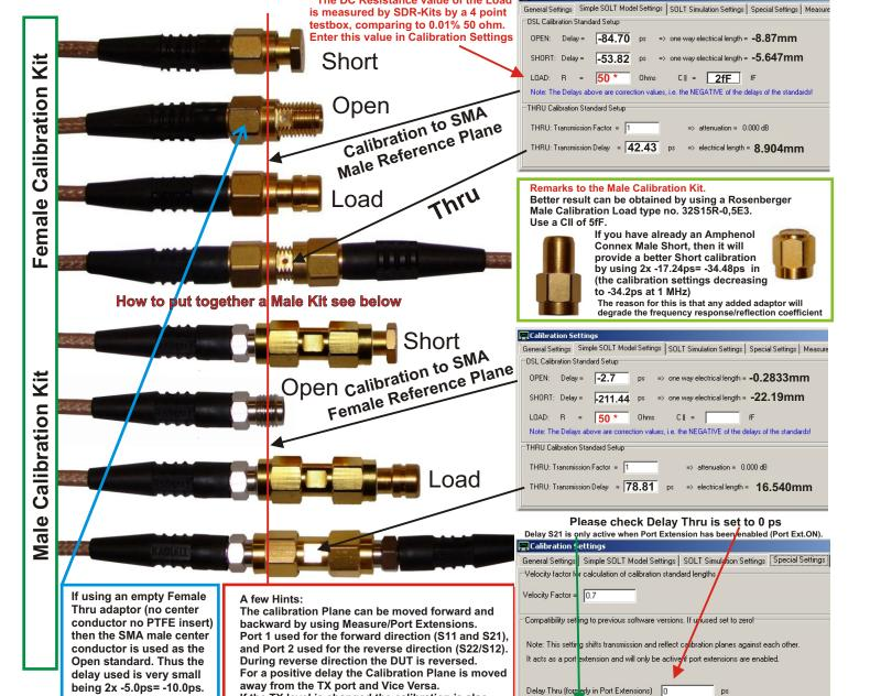
If the TX level is changed the calibration is also changed slightly. READ ALSO THE HELP FILE
