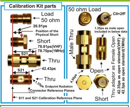
On this sheet you will find the settings required in "Calibration Settings" and "Arbitrary calibration" for the Reflection (S11/S22) and Transmission (S21/S12) calibrations.
