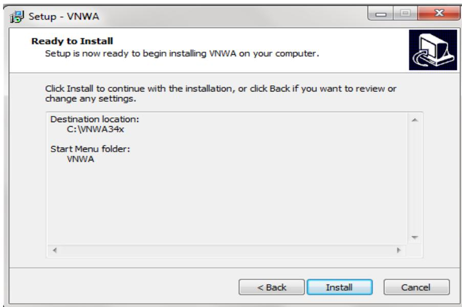
3.1.9 Press "Install" – VNWA Application and helpfile are now installed and Driver Installation window is displayed. **Note:** Do **NOT** plug-in VNWA at this time
