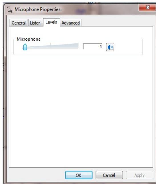
3.3.7 Check on VNWA Setup Screen that sinewave covers approx 50% to 60% as shown in step 3.3.6 and 3.3.7. If necessary adjust Microphone level until this is achieved.
