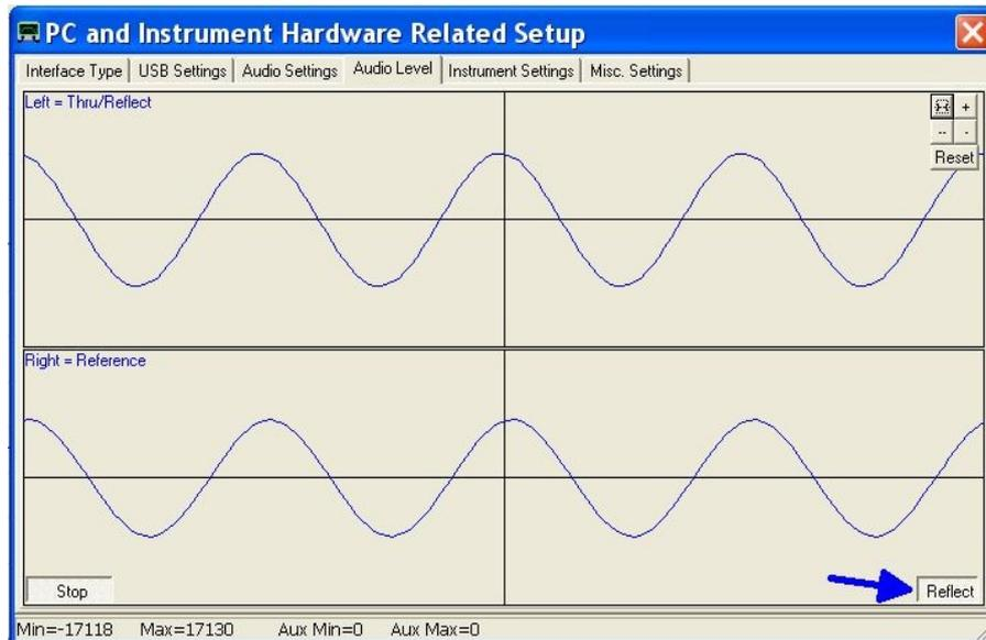
3.5.8 Connect the TX port and RX port with an SMA cable and check that Left Channel sinewave has disappeared (No signal reflected) . Now select “Thru” (by pressing on softbutton "Reflect" and check that the Left Channel sinewave is displayed as shown in screenshot below.
