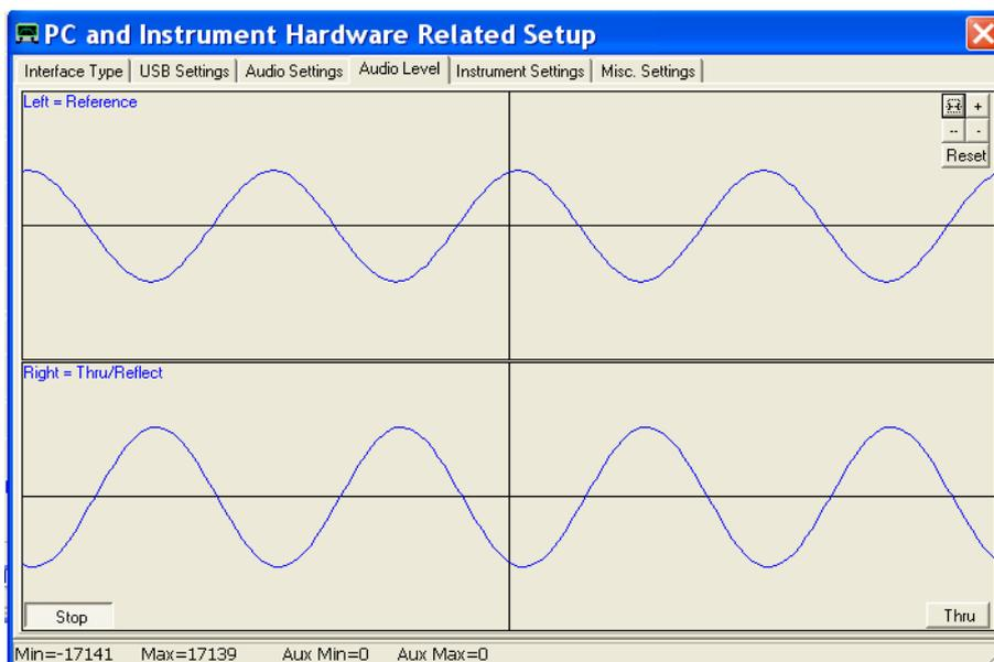
3.5.9 Click “Stop“ cease the Audio test. Next click on "Instrument Settings” and check whether clock is set to “auto”. Note that for VNWA 2, the clock is generally a little below 36 MHz, somewhere between 35.855 MHz and 36.000 MHz depending on Crystal fitted. When performing Audio test press ++ / + or -- / - buttons until the sinewaves are almost stationary on the screen. If you have a frequency counter perform Calibrate DDS Clock calibration as described in the VNWA helpfile
