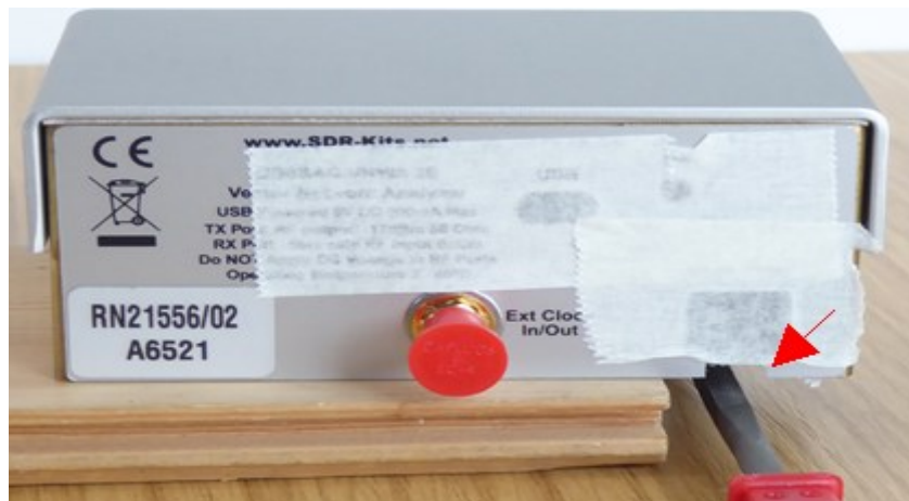
Red arrow in above image shows location slot and filing method to avoid PCB contamination
