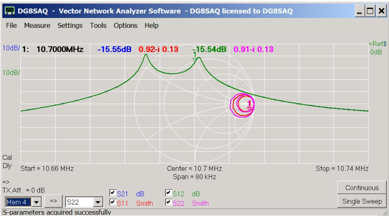
Note, that the forward Sparameters (S21, S11) might slightly change during the reverse measurement as the software uses the additional information of the reverse measurement to correct the forward measurement results in order to obtain the highest possible accuracy.
