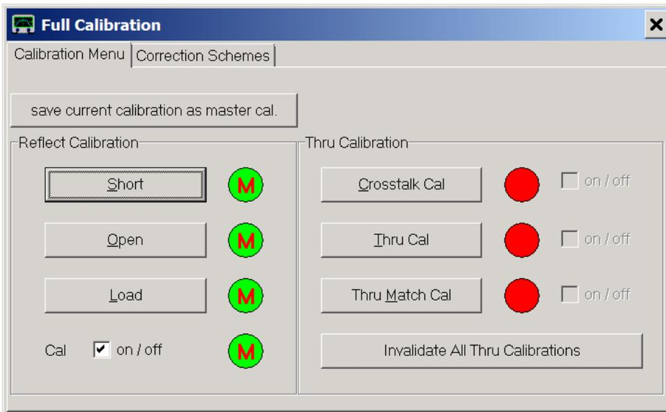
Next, we need to calibrate the VNWA for transmission. We therefore connect the test cable ends of TX port and RX port with the Thru standard...
