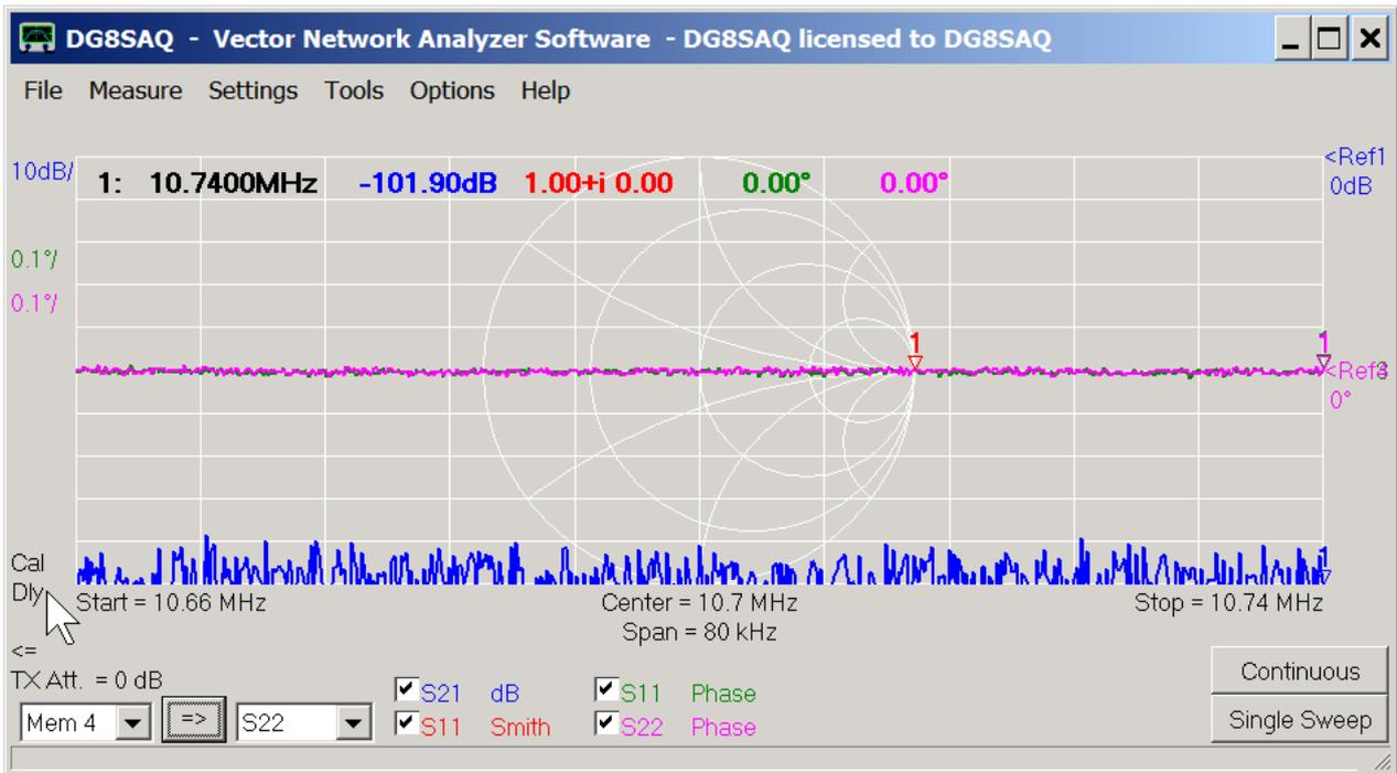
Note the labels Cal and Dly in above figure at the mouse arrow indicating that a calibration is active and port extensions (=port delays) are activated.
