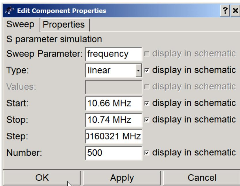
We use the same frequency grid as in our S-parameter file. Now, we can launch the simulation by pressing the **Simulate** button:
