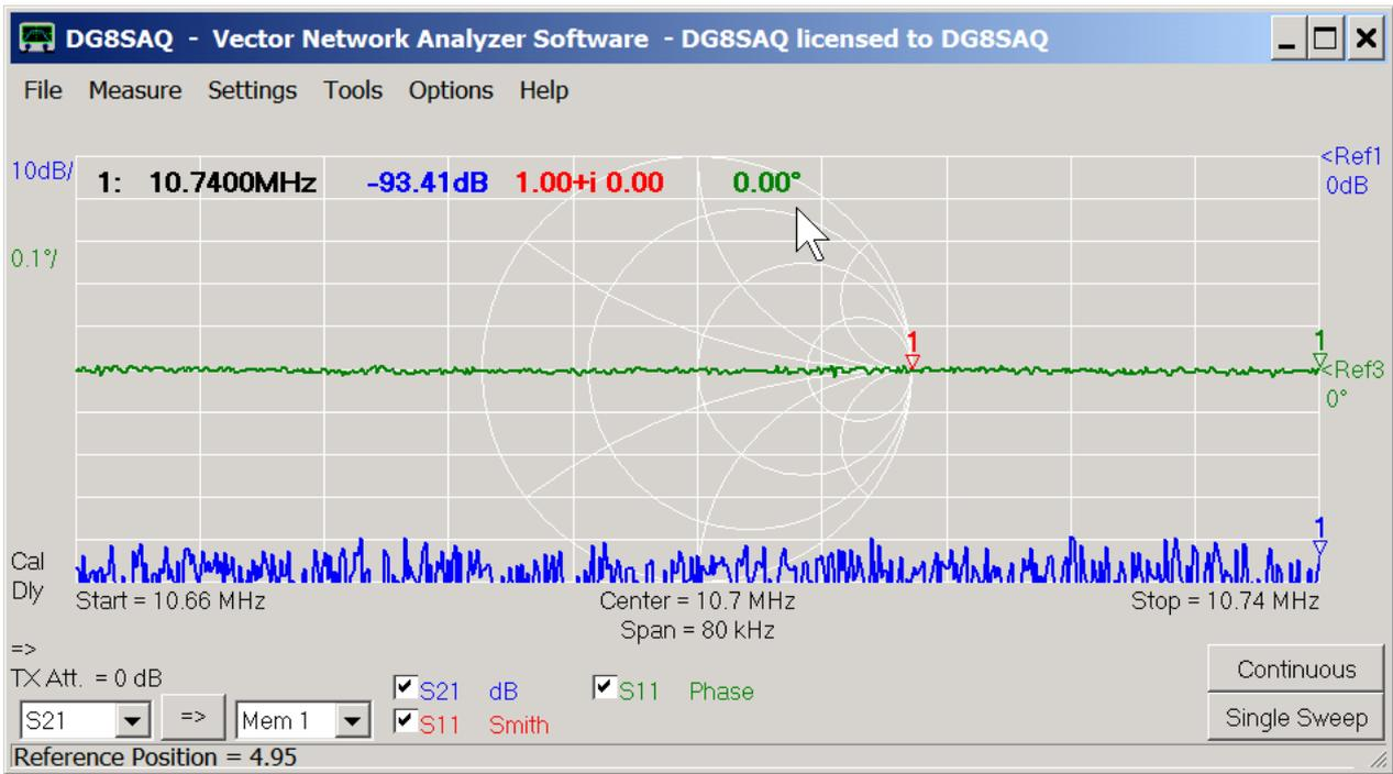
Note, that the reflection coefficient S11 is now exactly  $1+i0$ , which is the open reflection condition, corresponding to a dot at the right edge of the Smith chart.
