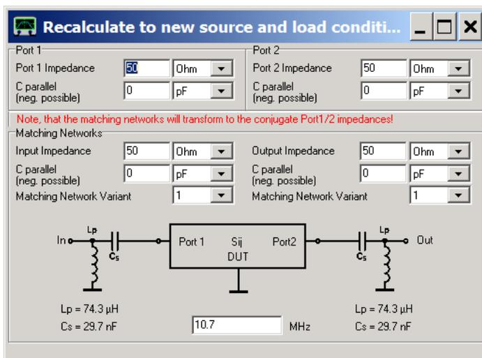
We can now modify port 1 and port 2 impedances by using the keyboard or the mouse wheel (right-click onto the edit fields to change the mouse wheel increments) and observe in the main window how the S-parameters change when transformed to different terminating conditions, e.g. changing the terminating impedances on both sides to 1550 Ohms
