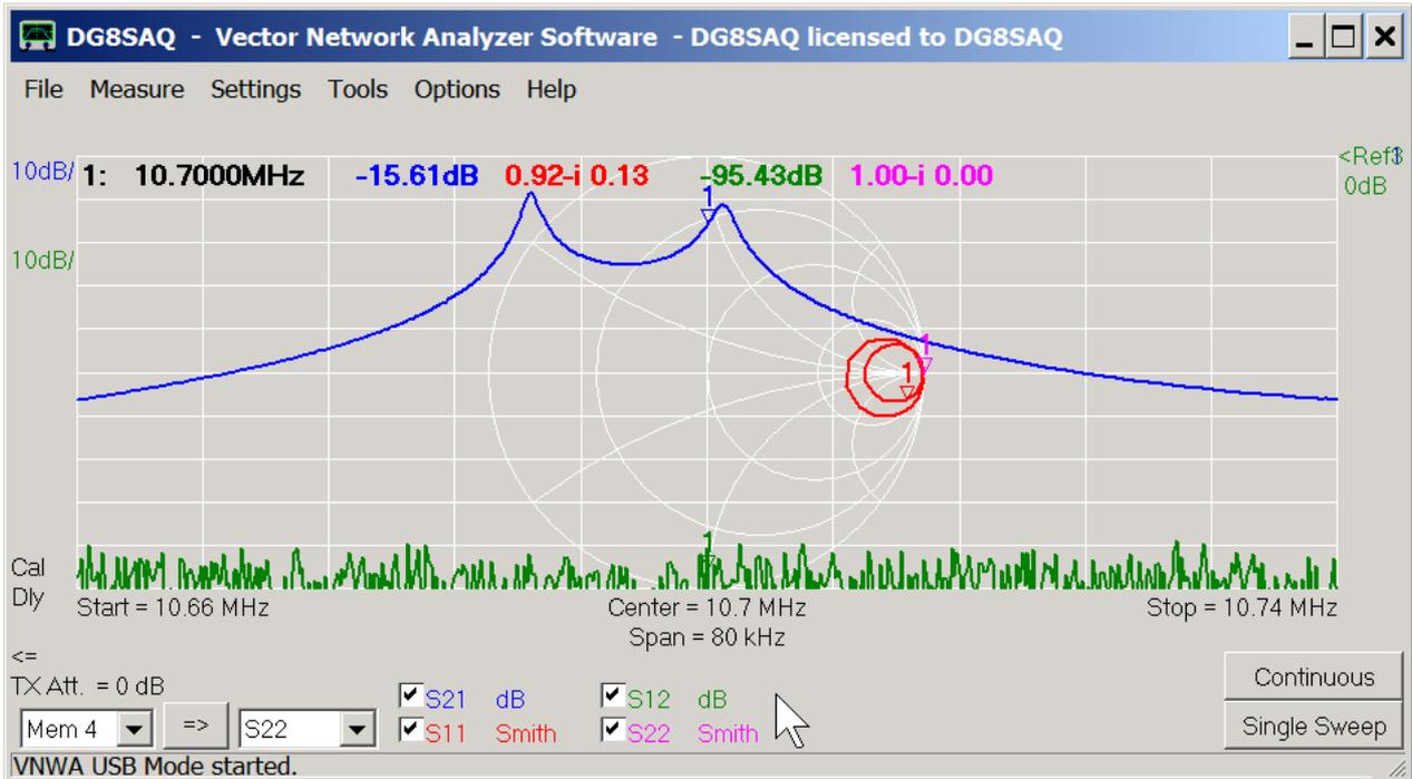
Note, that meanwhile we have chosen to display all four S-parameters S11, S21, S12 and S22.
