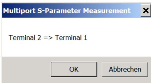
This means, that we have to reverse our test board, i.e. connect port 2 to the VNWA TX port and port 1 to the VNWA RX port:
