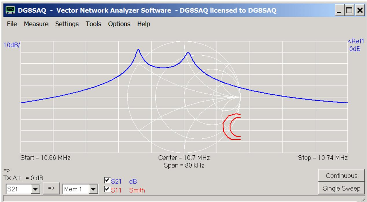
The just measured S11 reflection data is partly outside the Smith chart because our VNWA is not yet calibrated. The data is not valid yet.
