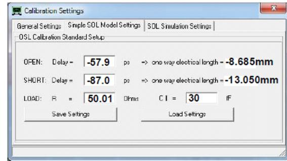
... which places the calibration plane exactly into the middle of the Thru calibration standard. The above calibration kit data was compiled by Kurt Poulsen and is available from his web page <http://www.hamcom.dk/VNWA/> also for different calibration kit builds and manufacturers.
