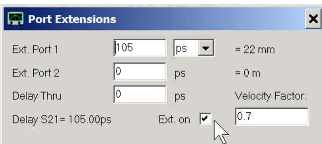
We check the **Ext. on** box (mousepointer) and set focus to the Ext. Port 1 by clicking on it. Next, while observing the green S11 phase trace in the main window, we turn the mouse wheel or edit the field until the the S11 phase is zero:
