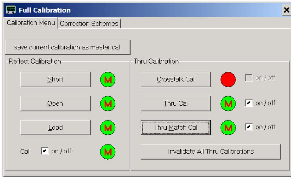
We close the calibration window and double-check the calibration by measuring the "Thru" calibration standard.
