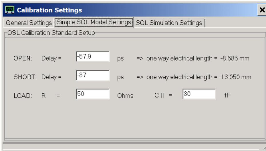
Note: Before performing any calibration measurement, make sure, that the instrument sweep rate is set to the lowest value you intent to use the calibration with, otherwise your later measurement results will be dominated by the noise of your calibration measurements. We have selected a total sweep time of 4s above which is as slow as we want to sweep, so we're ok.
