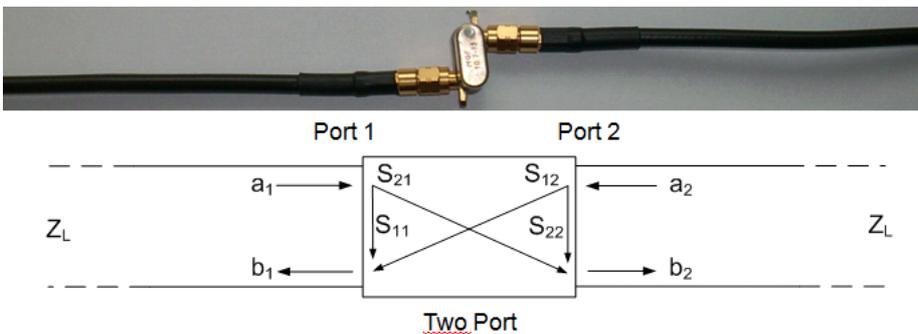
The complex wave amplitudes  $a_1$ ,  $a_2$ ,  $b_1$  and  $b_2$  are complex numbers that carry both the wave amplitude and the wave phase information.
