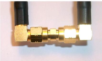
... and press the "Thru" button and let the instrument do the calibration sweep.
