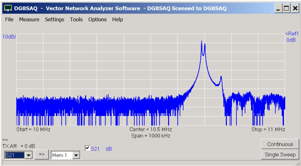
The span (1MHz) is much too high and the center frequency is off. We place a bandwidth marker by right-clicking onto the main grid in order to determine the optimum center frequency and span:
