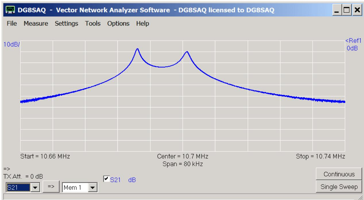
This way, we have a good view of the passband of the filter (between the two maxima) and we also see some of the nearby stopband. Note, that the filter passband is not flat, because the filter is not impedance-matched to the VNWA impedance level of 50 Ohms.
