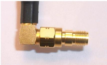
We select "Measure-Calibrate" or simply press the c-key on the keyboard, press the "Open" button, confirm that the open standard is connected and observe the instrument measuring the standard. When the measurement is completed, the red Open light turns green:
