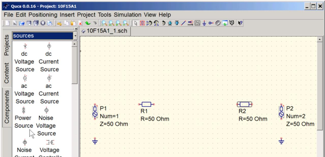
Then, we switch to **file components** and add a **2-port S parameter file** component (and from the lumped components another ground component which we have previously forgotten) :
