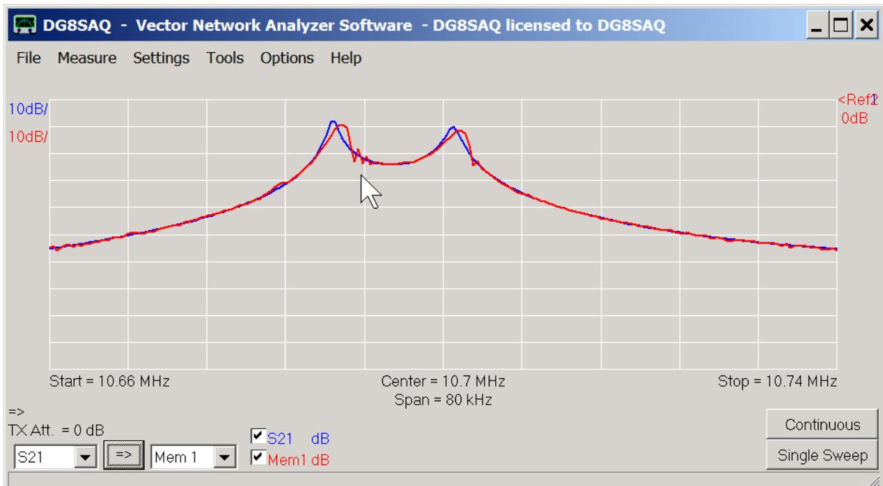
Clearly, the red trace was taken at a too high sweep rate as the maxima are shifted to the right and the filter is ringing after the maxima (marker arrow).
