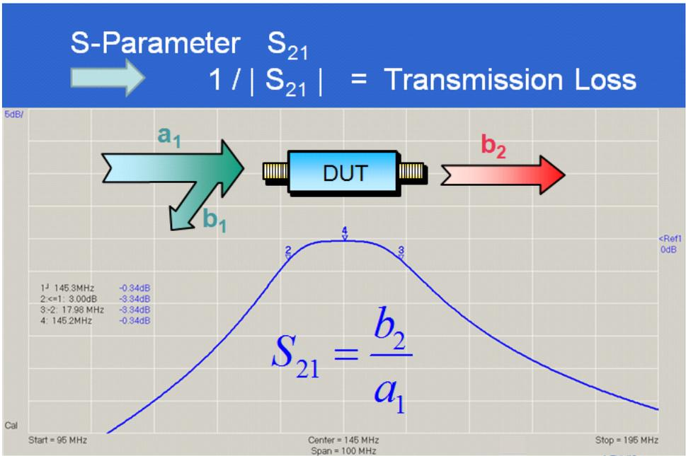
The inverse of  $|S_{21}|$  is known as transmission loss. For example, a 10dB / 50 Ohms attenuator will show  $S_{21} = -10\text{dB}$ .
