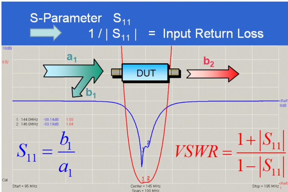
The inverse of the magnitude of  $S_{11}$  is known as input return loss. I.e. a device showing a return loss of 10dB will yield  $|S_{11}|=-10\text{dB}$ . This means, the reflected wave is 10dB weaker than the incident wave or 1/10th of the incident power is being reflected. But, since  $S_{11}$  also carries the phase information, also the input impedance of our DUT can be calculated from  $S_{11}$ .
