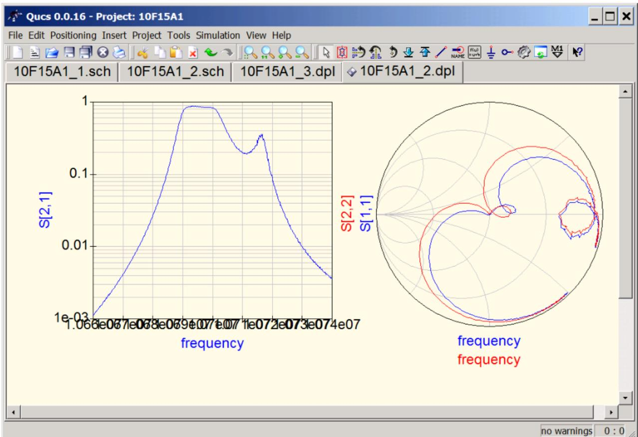
We add a capacitor to the internal filter connection to improve the match:
