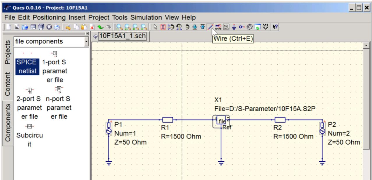
The schematic is done. It looks like the hardware in our previous measurement. Now, we have to tell the simulator what kind of simulation we want. We change to the **simulations** components and add an **S parameter simulation**:
