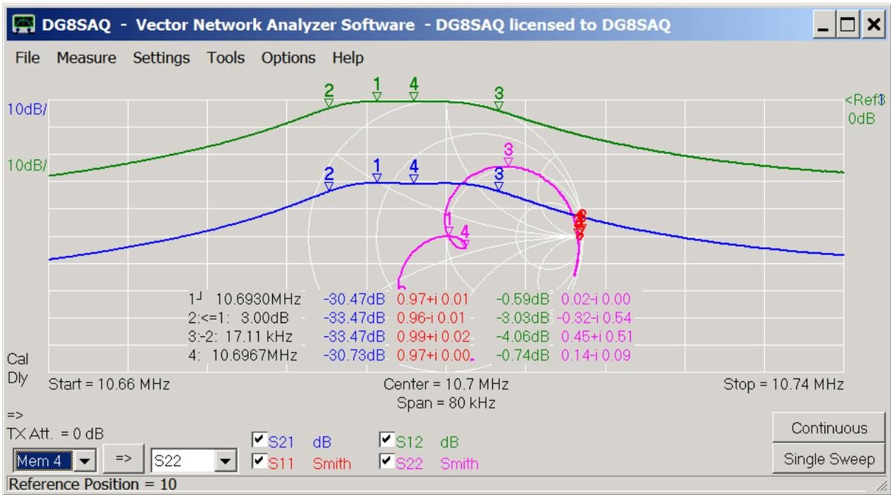
Indeed, the filter passband is flat now, but the insertion loss has increased by about 30dB in comparison to our S12 trace which has survived from our software matching experiment!
