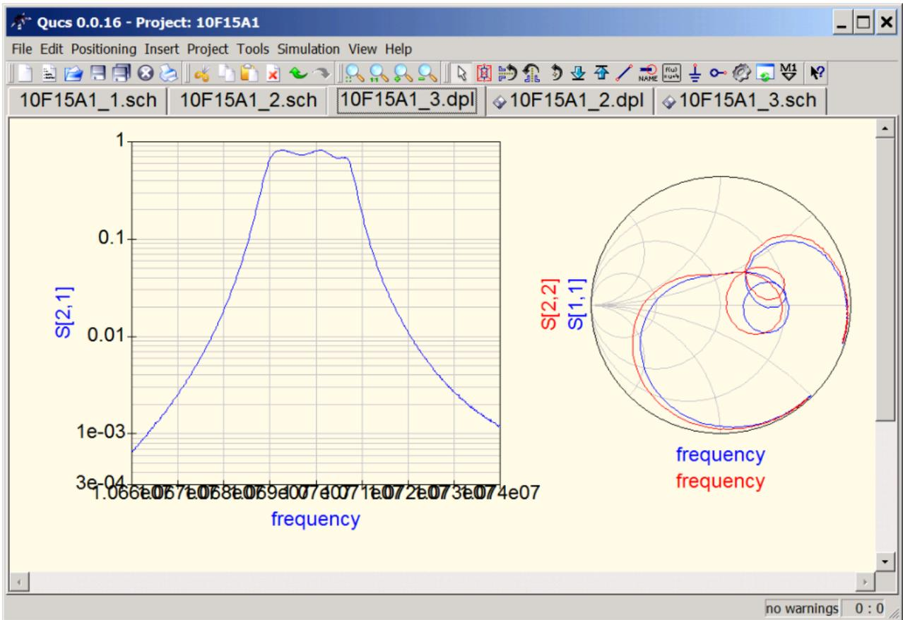
We could easily continue to optimize internal and external matching and thus design a perfect four pole crystal filter. Obviously, a simulator like QUCS together with the VNWA for acquiring S parameter data is a powerful pair for RF design.
