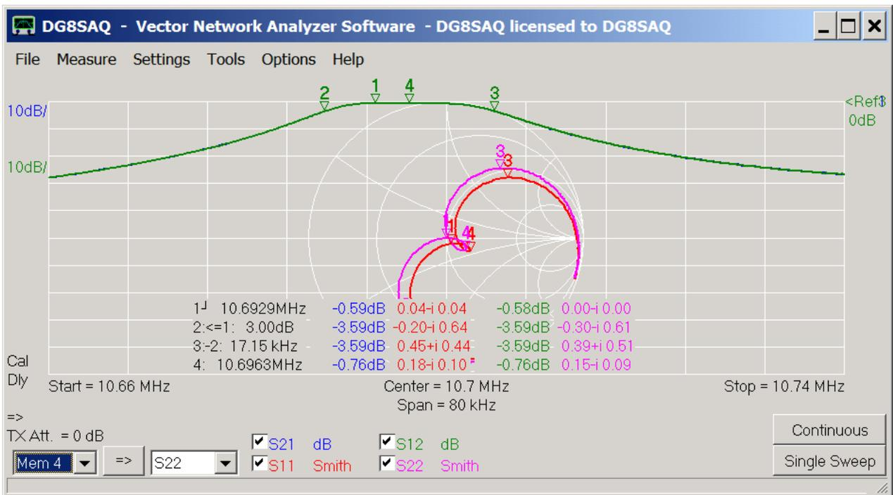
We can easily implement this impedance condition in an experiment by connecting 1500 Ohms resistors in series with the VNWA RX and TX ports. The RX and TX port impedances of 50 Ohms will add to these 1500 Ohms to yield 1550 Ohms impedance at the filter:
