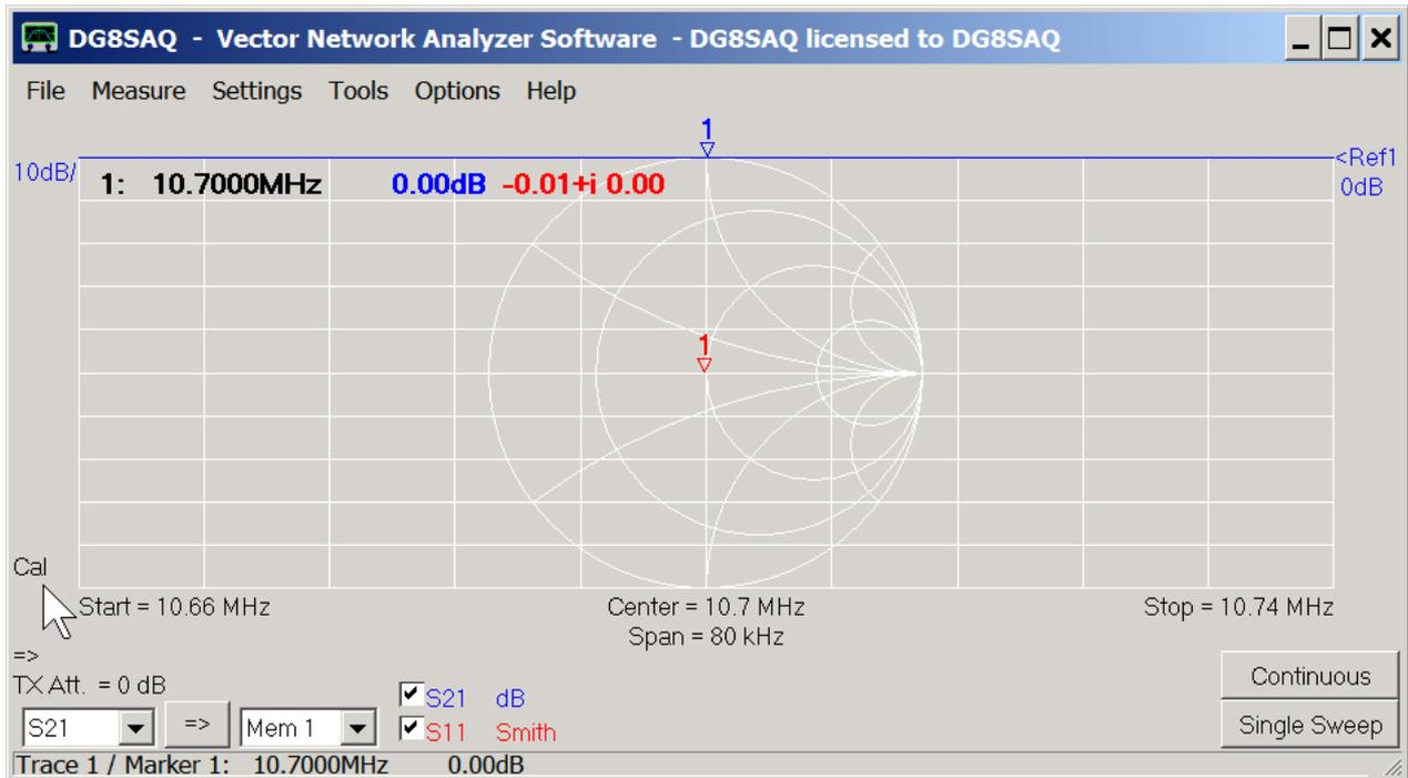
As our Thru standard has by definition 0dB attenuation, we obtain the flat blue 0dB line. We have also measured the reflection coefficient of the RX port (red trace reduced to a dot, barely visible without marker), which is very close to zero for all frequencies.
