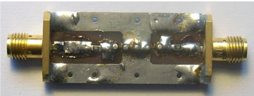
We connect the modified test board with the crystal filter to the VNWA and do a single sweep in forward direction using the original calibration and settings from the S-parameter measurement:
