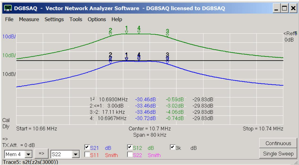
For clarity, we have reverted to the original scales 10dB/ and a unique reference level of 0dB on top. We can read off the black 3k simulation trace, that 3000 Ohms will introduce an extra loss of 29.83dB, which looks about right compared to the blue S21 trace.
