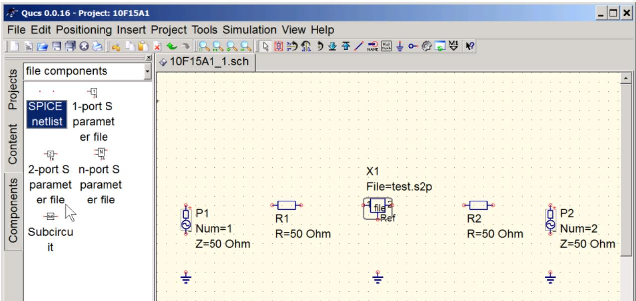
We need to change our resistors to 1500 Ohms, therefore we right-click the resistors and select **Edit Properties**:
