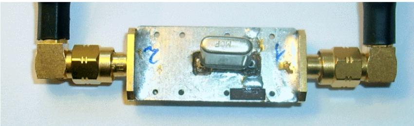
Once we are done with reconnecting the test board, we press **OK** on the multiport assistant and observe S12 and S22 being measured:
